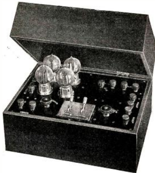
This is a Power Amplifier Used to Boost up the Current of a Microfone Circuit in Order to Operate a Telemegafone at Maximum Efficiency.
