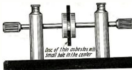
Here is a Cheap and Efficient Quencht Gap for Those Who Still Use a Spark Coil.
