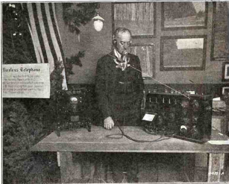
On the left, the fotograf shows the complete radiofone set used in detecting and reporting fires occurring in the forests. Thanks to these apparatus the fire-fighting squads may promptly be notified and directed right to the fire.
