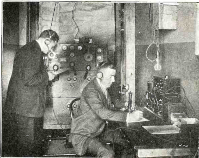
Inside View of the Radio Station Installed in Hoboken, N. J. for the Broadcasting of the Results of the Dempsey-Carpentier Fight. In the Background May Be Seen the 3 K.W. Radiofone Set With the Operator Speaking Into the Microfone.
